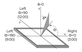
Figure 4. The definition of viewing angle
