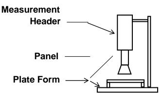
PR-670 / MINOLTA CS-100 Color Analyzer
