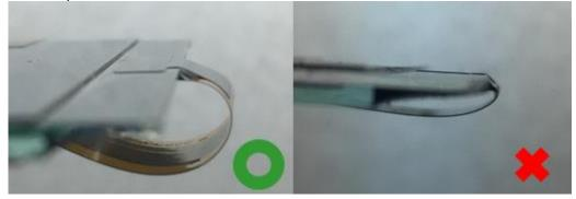
Avoid bending the film at IC bonding area. It could damage the IC ILB bonding. It should avoid bending the IC seal area. Please keep the bending distance >1.5mm.
