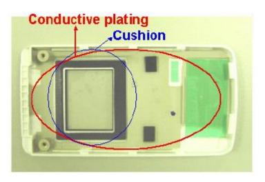
It is recommended that a plating conductive layer be used in the housing for EMI/EMC protection. And, the enough space should be reserved for the IC placement if the IC thickness is thicker than the TAB film when customer design the PCB.
