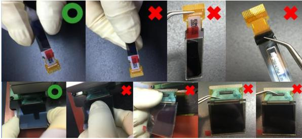
7. Use the tweezers to open the clicks on the connector of PCB before the insertion of FPC/COF, and click them back in. Once the FPC/COF sits properly in the connector, use the tweezers to avoid the damages.
