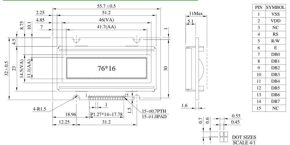
The non-specified tolerance of dimension is  $\pm 0.3 \mbox{ mm}$  .
