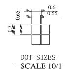
The non-specified tolerance of dimension is  $\pm 0.3 \text{ mm}$ .
