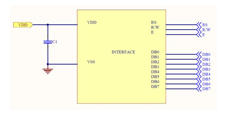
Pin connected to MCU interface: RS, R/W, E, DB0~7
