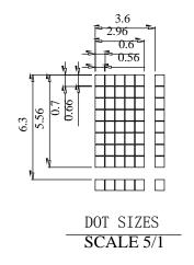
The non-specified tolerance of dimension is  $\pm 0.3\ mm$  .
