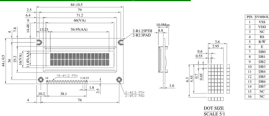
The non-specified tolerance of dimension is  $\pm 0.3 \text{ mm}$ .
