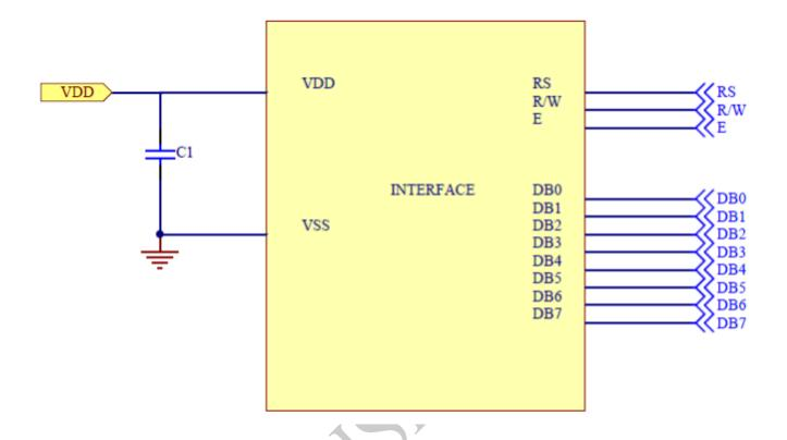
Pin connected to MCU interface: RS, R/W, E, DB0~DB7
