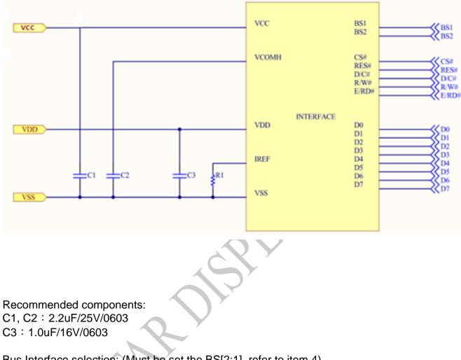
Bus Interface selection: (Must be set the BS[2:1], refer to item 4) 8-bits 6800 and 8080 parallel, SPI, I2C
