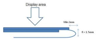
(12) The module should be fixed balanced into the housing, or the module may be twisted.
