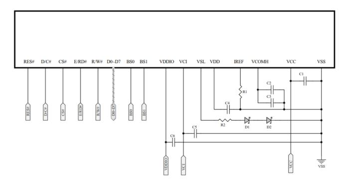
R2 = 50Ω, 1/8W D1, D2= 1N4148 C1, C2=4.7uF C3=0.1uF C4, C5, C6=1uF
