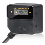
The RT242 series fixed mount scanners are outstanding at **super thin design**: only 2cm in thickness. In addition, they are also easy mounting designed, with a bracket available optionally; and also powered with high-performance scan engine inside, which enables them to read most 1d and 2d bar codes excellently.
