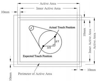
X direction of linearity:  $\Delta x/X *100\%$ . Y direction of linearity:  $\Delta y/Y *100\%$ .
