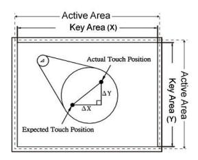
X direction of linearity:  $\Delta x/X *100\%$ . Y direction of linearity:  $\Delta y/Y *100\%$ .
