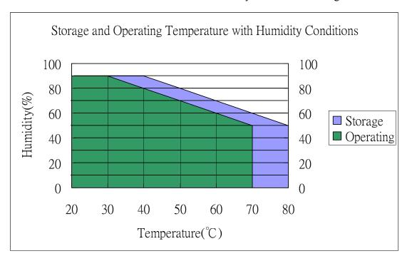
Fig.5 Storage and Operating Temperature with Humidity Conditions
